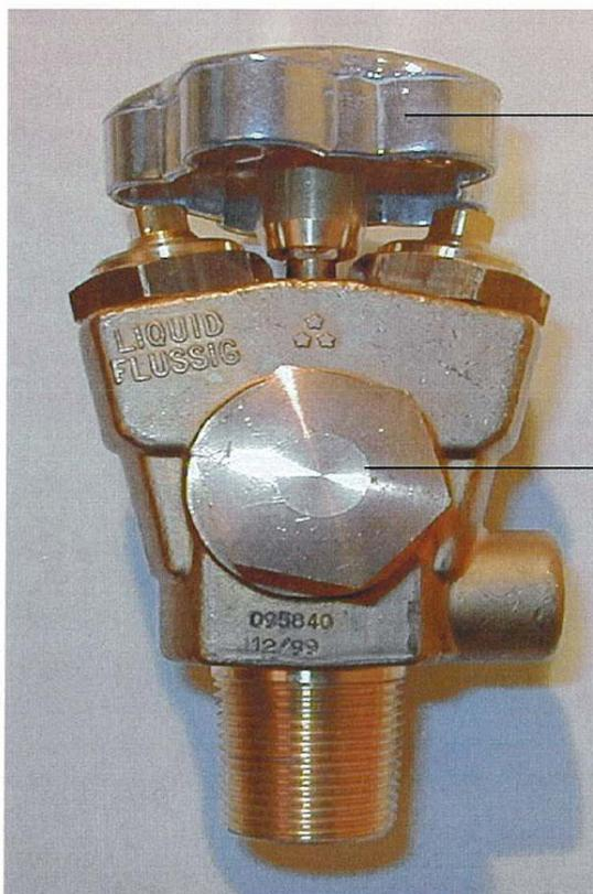
Handwheel located on central "transit" spindle
