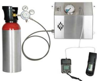
The BTS-X is the newest product for bump testing or calibration testing hand held gas detectors. Completely pneumatic, the BTS-X operates using the calibration (test) gas. With no batteries or mains power the BTS-X can be located anywhere in the water or wastewater treatment facility.
